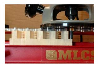
Install the angled-finger "pins" template onto the jig and let it lay directly on top of the backer block scrap piece clamped under the top clamping bar.
